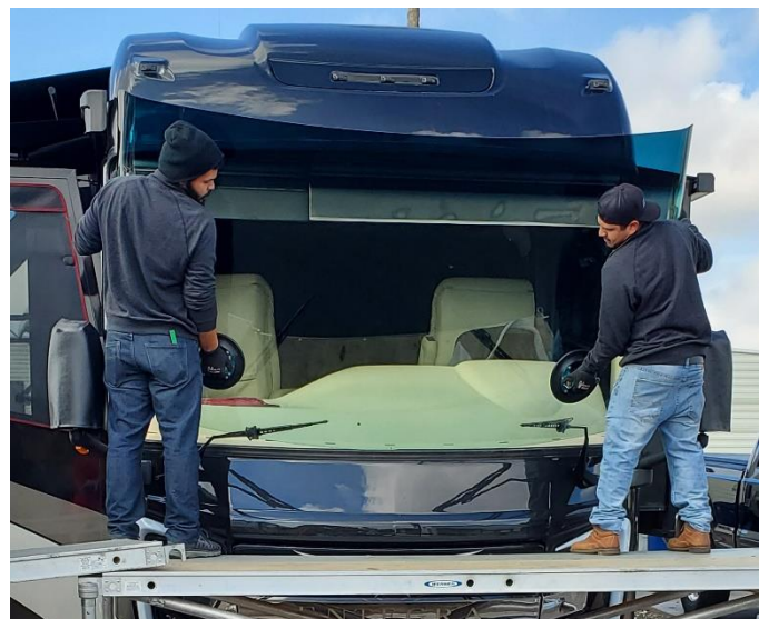
Placing the new windshield was done carefully making sure everything was lined up properly.
